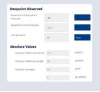
We also supply a handy, portable pressure dew point calculator with every dew point meter and hygrometer. Especially practical when you are onsite taking spot check readings and your dew point reading requires conversion to an alternate measurable value. To find out how to use this pressure dew point calculator, follow our <u>step-by-step guide</u> or watch the <u>video tutorial</u>.
