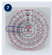
Rotate the alignment arrow to the °C reading in step 5, e.g. -17.5 °C. You will find the conversions for the following units: °F, g/m³, lb/MMSCF, ppm(V) and ppm(W).
