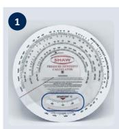
After taking a reading with your dewpoint meter (we used the SADP), rotate the centre wheel [B] to match the dewpoint shown on the instrument. We will use -40 °C for this example.
