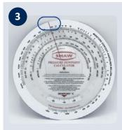
Hold the alignment arrow [C] and the moisture content value in a fixed position, rotate the centre wheel [B] to change the pressure.
