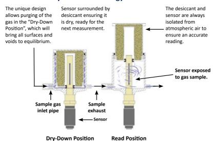
Keeping the sensor dry between tests ensures that the SADP is ready to carry out rapid spot checks. The unique design of the desiccant head achieves this by surrounding the sensor with desiccant, keeping the sensor dry. The head is then lifted for sampling, exposing the sensor to the sample gas.
