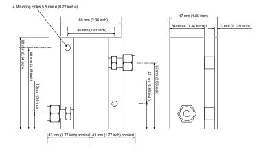
NOTE: The assembly is shown with  $\frac{1}{2}$  inch OD tube fittings. The dimension across the tube fittings will vary for all other size fittings
