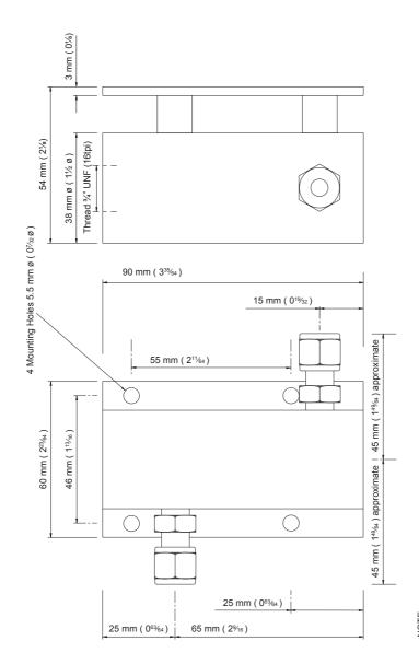
The assembly is shown with 6.35 mm (1/2 inch) OD tube fittings. The dimension across the tube fittings will vary for all other size fittings.
