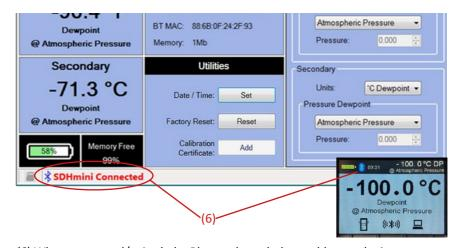
(6) When connected/paired, the Bluetooth symbol turns blue on the instrument.
