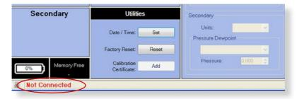
Always ensure the USB cable/Bluetooth is connected to the instrument and PC when working in the *SHAW SDHmini User Tool* software. If you have not connected the unit to the PC and attempt to start using the *SHAW SDHmini User Tool* software it will show a "Not Connected" message.
