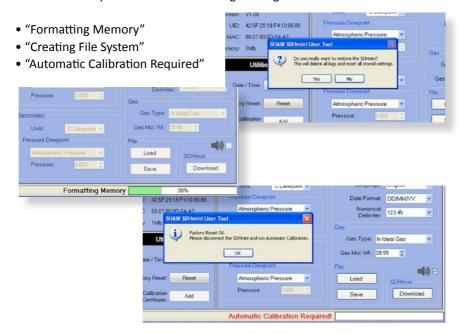
**Warning:** Performing a *factory reset* will erase all saved settings and data and default the following to factory settings: date format, language, main display units, secondary display, gas weight, gas type, AutoCal value, location ID, numerical delimiter.
